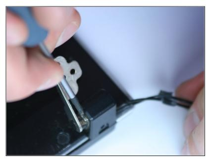
• Remove the small enclosures around the hinges.
