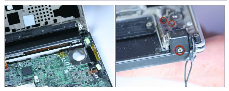
• Remove the six screws (three on each side) holding the top panel of the chassis to the display with a Phillips #0 screwdriver.
