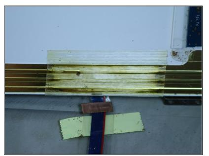
• Remove the tape holding the cable to the screen.
