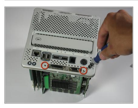
Remove the screws on the back of the VGA port.
