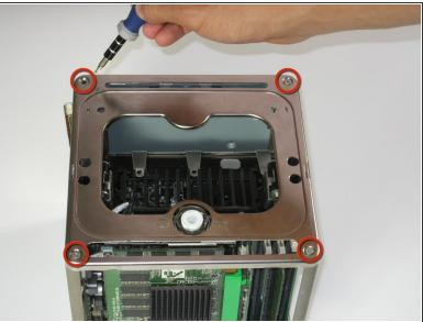
Place the cube upside down and remove the four T10 Torx screws on the front plate. Then remove
