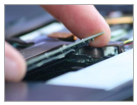
After the ram has sprung up, carefully grab the edges with your fingers and gently pull straight out.
