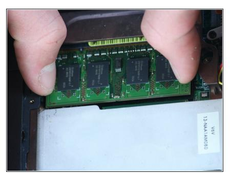
Carefully use your thumbs to push out the metal tabs and the RAM should spring up.
