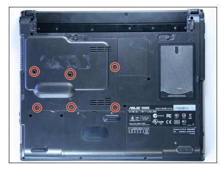
On the back panel unscrew highlighted screws and carefully put them to the side as not to lose them.
