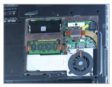
Locate the RAM chip and the two metal tabs holding it in place.
