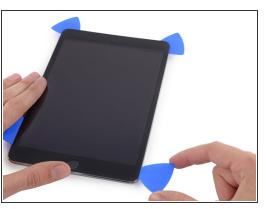
Continue to slide the pick down the right edge of the iPad, releasing the adhesive.
