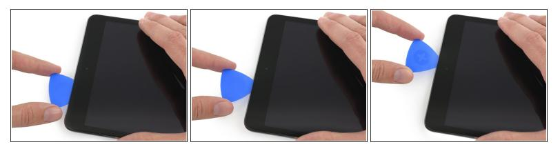
Pull the pick out slightly, and slide the very tip gently along the top of the front-facing camera section of the top edge.
