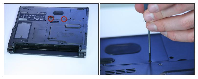
• Remove the two screws using a Phillips #0 screwdriver.
