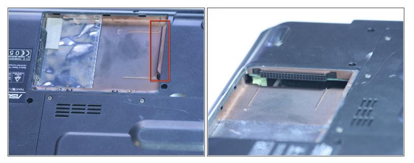
The highlighted area is where your hard drive would be. Slide it out away from its slot and pull it gently to remove.
