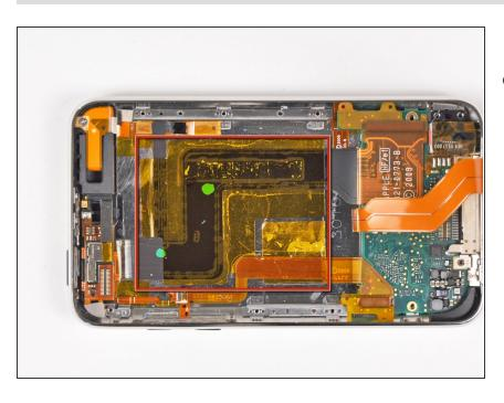
Carefully remove the two large pieces of tape securing the ribbon cables to the rear panel.
