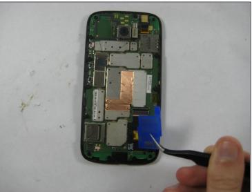
Remove the plastic protective cover by using the tweezers.
