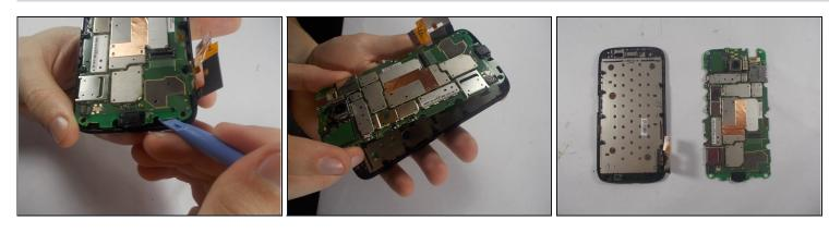
• Use the plastic prying tool and slowly work around the edges of the phone to detach the screen from the motherboard.
