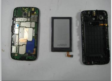
• With the battery already disconnected, work around its edge with the pry tool to remove it from the assembly.
