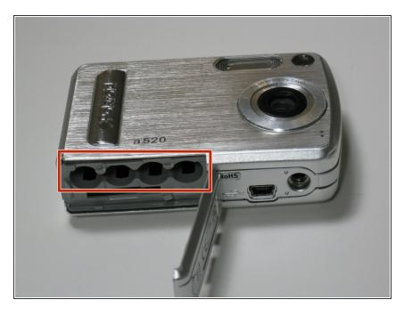
Remove the batteries from the camera.
