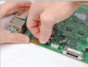
Disconnect the optical drive power and SATA cables from the motherboard.
