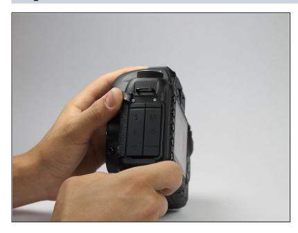
Peel back the rubber cover above the in/out ports to reveal two screw heads.
