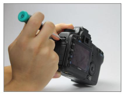
• Remove both 5.4 mm screws using a Phillips #0.
