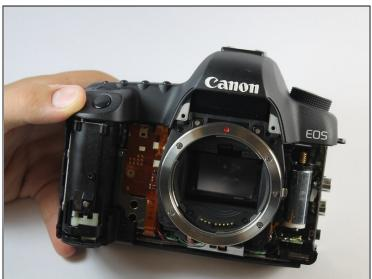
• Remove the front panel by lifting upwards from the right side where the in/out ports used to be.
