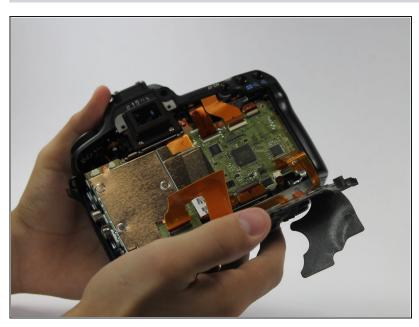
The back panel can now fall off easily by turning the device upside down. Be sure to catch it so the data ribbons do not tear or tug.
