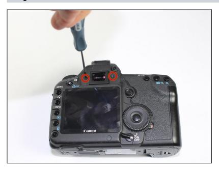
Remove each 6.3 mm screw on either side of the viewfinder using a Phillips #0 screwdriver.
