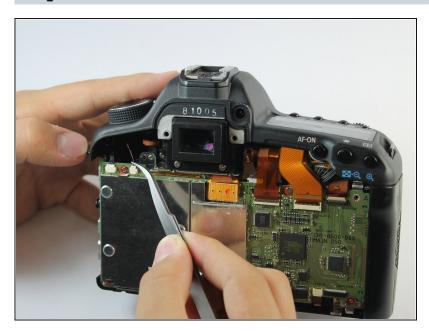
Using <u>tweezers</u>, pull out the wire attaching the front panel to the motherboard.
