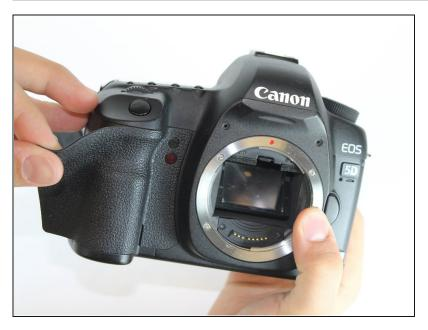
Peel off the rubber cover on the front panel in order to access the screws underneath.
