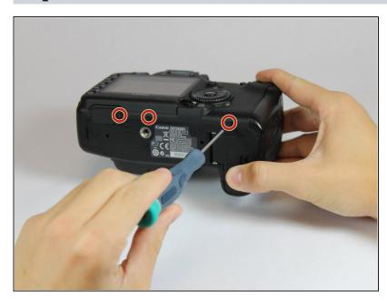
Remove the three 4.8 mm screws on the bottom of the back plate using a Phillips #0.
