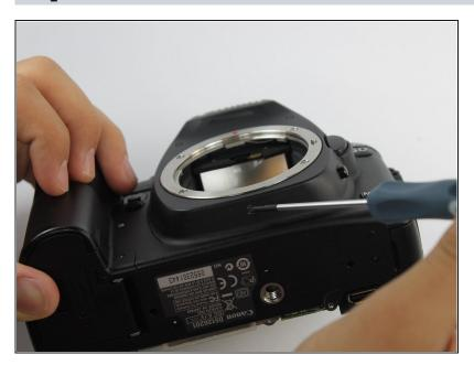
Remove the single screw underneath where the lens would be using a Phillips #0.
