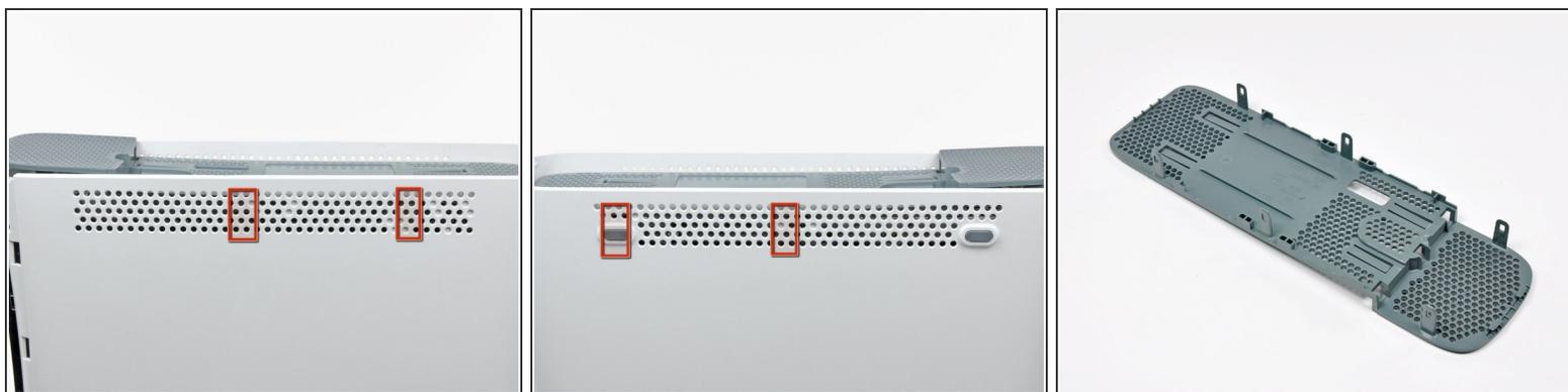
**i** In the next few steps, you will use the tip of a spudger or the finger of an Xbox 360 opening tool to release the clips along the left and right sides of the top vent. Their locations are highlighted in red.
