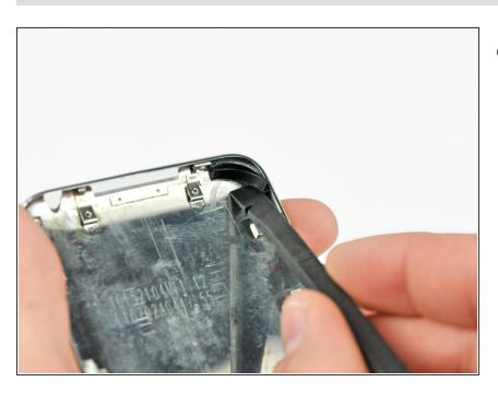
Use the flat end of a spudger to pry the protective rubber grommet from the bottom left hand corner of the rear panel.
