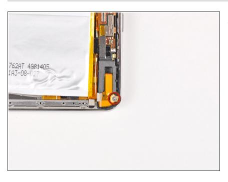
Remove the remaining Phillips screw securing the upper logic board to the rear panel.
