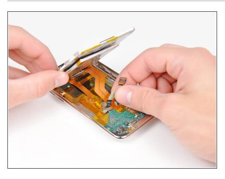
Peel the display data cable off the adhesive securing it to the rear panel.
