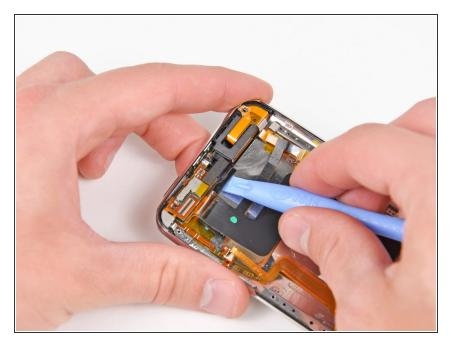
Use an iPod opening tool to pry the black plastic frame under the upper logic board up from the adhesive securing it to the rear panel.
