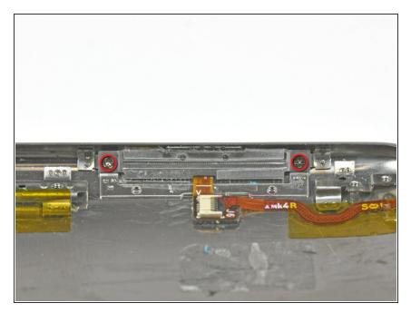
Remove the two Phillips screws securing the power/volume controls to the rear panel.
