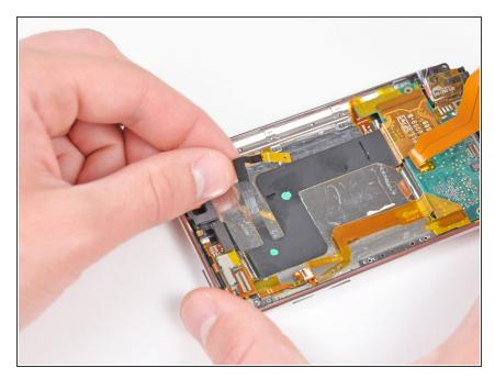
Carefully peel the antenna cable off the adhesive securing it to the rear panel.
