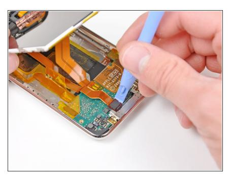
Use an iPod opening tool to pry the display data cable connector up off its socket on the logic board.
