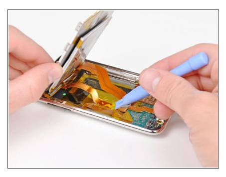
Use the edge of an iPod opening tool to remove the piece of tape covering the display data cable.
