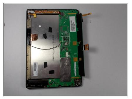
flip center chassis so that the back of the screen is facing you, and the hole is positioned in the bottom right corner.
