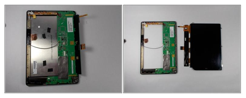
• Lift motherboard away from the screen. Pull frame off of the screen.
