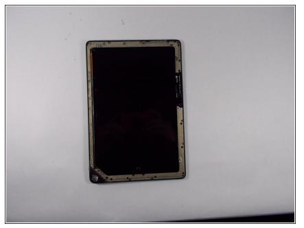
Remove every visible screw tying the chassis to the bottom frame using the T-4 attachment for the screwdriver in the iFixit screwdriver kit.
