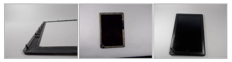
• wedge the plastic opening piece underneath the bottom left hand corner of the front frame. Pry the frame off of the Nook.
