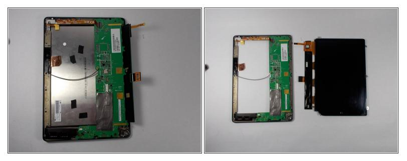
• Put the new screen back into place in the frame (the reverse of step 9). Place motherboard back into place on the back of the screen. And follow steps in reverse order to reassemble.
