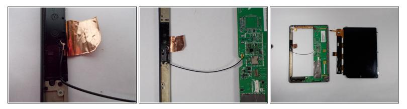
• Remove copper tape above the antenna, 3 quarters of the way up the left side of the nook.
