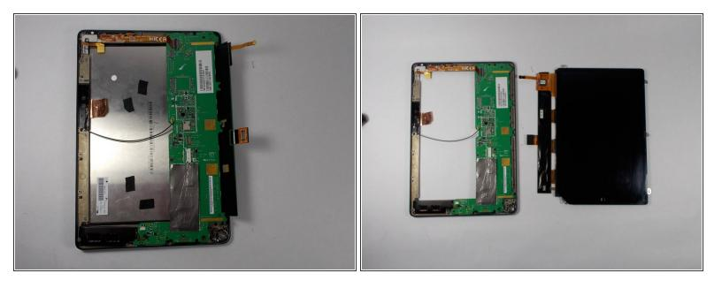
• Locate the foam covered orange strip on the motherboard. Pull up (away from motherboard) so that it i no longer connected to the motherboard.
