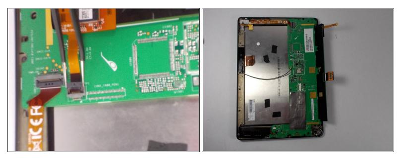
• Locate thin orange strip on the top side of the motherboard. Apply tweezers to the black casing that locks it into the motherboard (plastic piece will completely come out).
