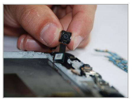
Replace the original camera with the new camera. It should come right out.
