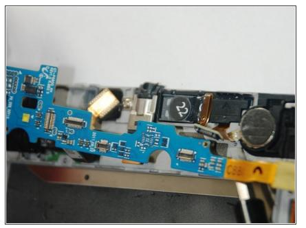
• Detach all ribbon cables from the flex cable, unscrew the flex cable, and remove the flex cable. This needs to be done in order to remove the camera which sits underneath the flex cable.
