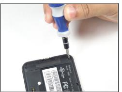
• Remove the thirteen 3.6 mm screws using the torx T5 bit in the screwdriver.
