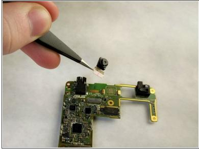
Use the tweezers to gently pull on the connector to remove the camera.
