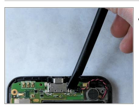
Using a spudger, pry the vibration motor connector from the motherboard.
