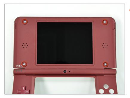
• Remove the four 3.5 mm silver Phillips screws securing the rear bezel to the front bezel.
