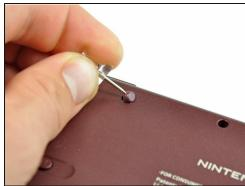
• Remove the four rubber screw covers on the lower case by prying them up with a push pin.
