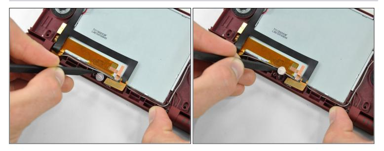
• Use the tip of a spudger to lift the microphone from its seat on the front display bezel.
