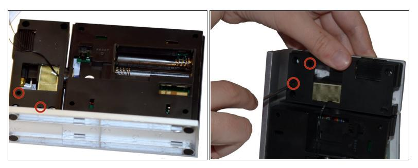
• Use a Phillips #00 Screwdriver to remove two (2) screws from back of projection arm.
