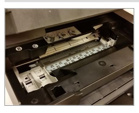
Inspect the printer thoroughly to ensure that all pieces of paper have been removed.
