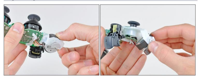
• Carefully push the two vibration motors out of the input board frame.
