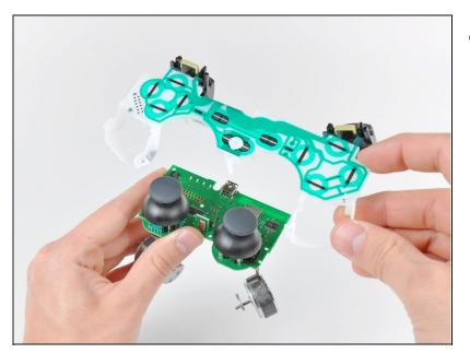
• Lift the input board assembly off the motherboard.
