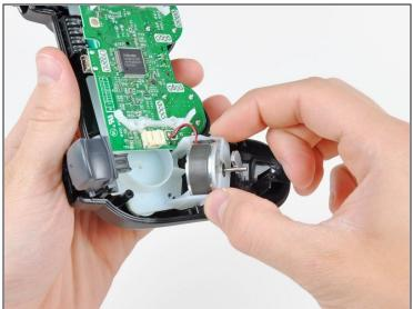
• Pull the vibration motor retainers away from the front cover to dislodge the motherboard assembly.
