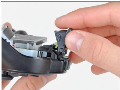
When reinstalling the #2 trigger, be sure the spring is positioned as shown before popping the axle back into place.
