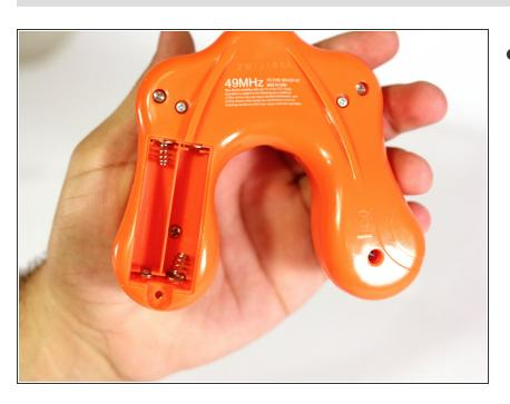
Remove the 2 AA batteries.
