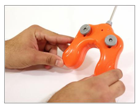
Turn the controller over to the backside and locate the battery cover screw.
