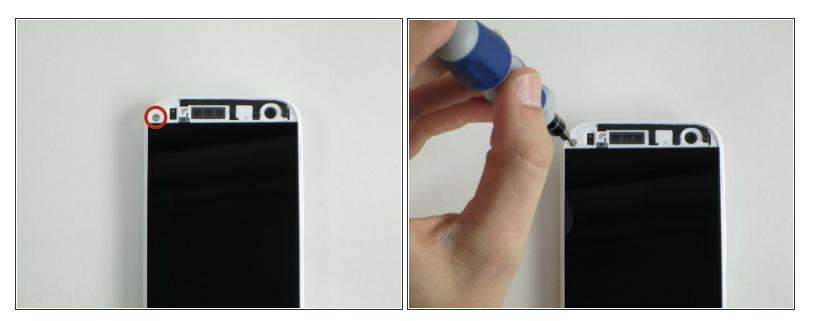
Remove the 2mm screw with a T5 torx screwdriver head from the iFixit tool kit.
