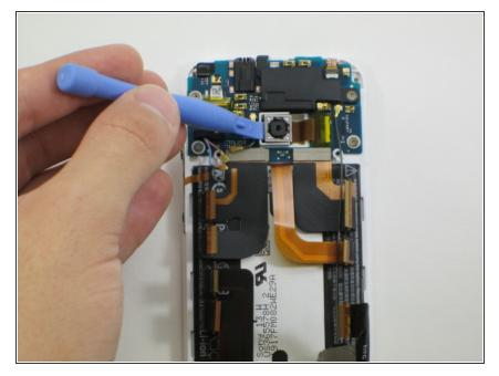
• Using the narrow pry tool, pry the rear camera loose from the frame.
