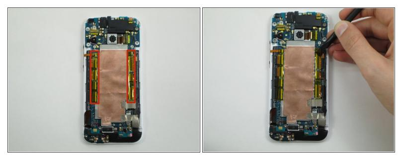
• Peel off the long yellow pieces of tape on the right and left side of the copper plate.
