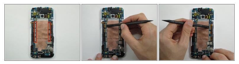
Using the flat end of the spudger, pop up the white tabs on all ribbon cable connectors located to the left and right of the copper plate.
