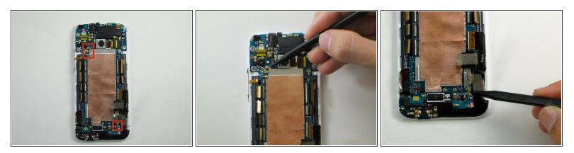
Use the pointed end of the spudger to pop off the four antenna connectors. Three are located on the top left corner of the motherboard and one on the bottom right.
