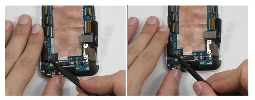
Using the pointed end of the spudger, pull the wires for the rumble motor to the left to pull the connector out of the board.
