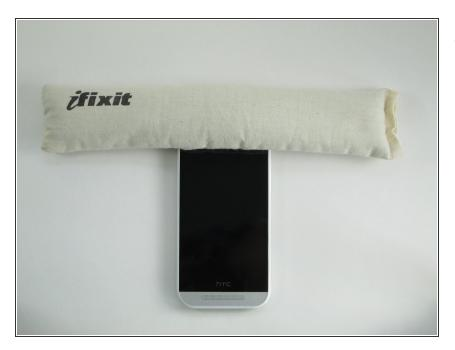
Heat up the top grey speaker plate with the iFixit iOpener for two minutes.
