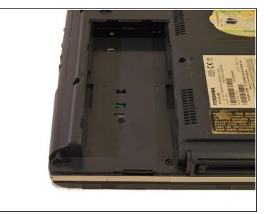
Lift the battery straight up, out of the computer.
