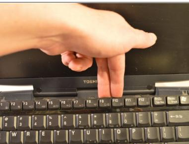
Lift the keyboard by holding the middle top of the keyboard.
