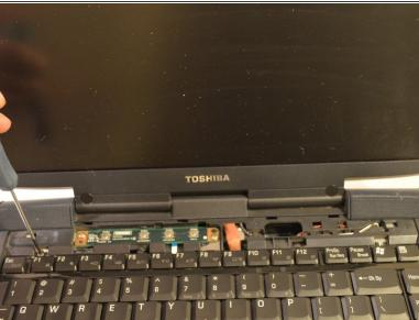
Unscrew the two screws near the top of the keyboard.
