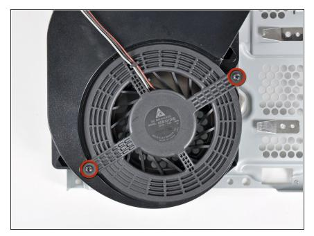
Remove the two 9.5 mm Phillips screws securing the fan to the heat sink.
