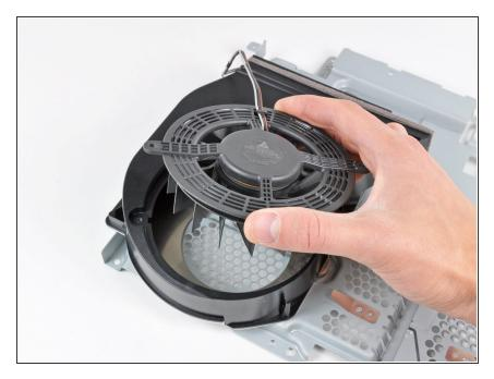
Remove the fan from the heat sink, minding the cables that may get caught on the fan shroud.
