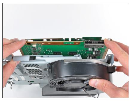
if necessary, gently pry the motherboard off the top shield near the heat sink and its shroud.
