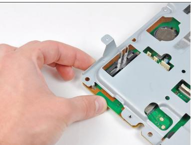
Gently press the board away from the top shield assembly near the fan connector and the corner of the board near the wireless sockets.
