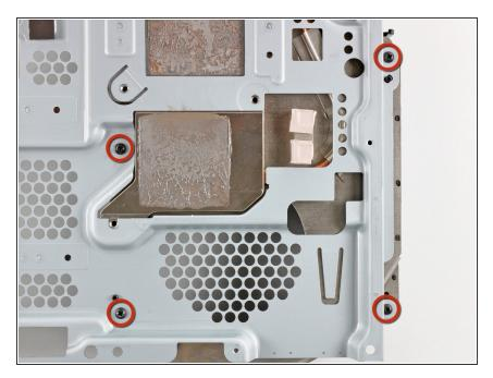
Remove the four 9.5 mm Phillips screws securing the heat sink to the top shield.
