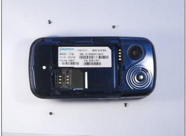
• Use a PH000 screwdriver to remove the four 2 mm screws from each corner of the device.
