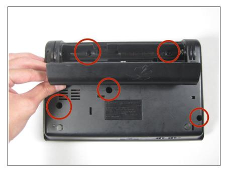
Remove the 5, 5.95mm screws as indicated in the picture.
