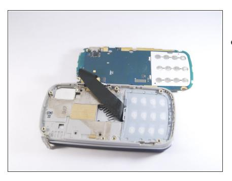
• Carefully lift up the motherboard to expose the back of the keypad.
