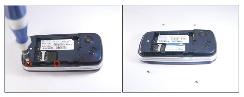
Use a Phillips screwdriver to remove the four 2mm Phillips #000 screws from each corner of the device.
