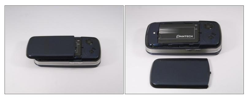
• Gently slide the backside phone cover off exposing the battery underneath.
