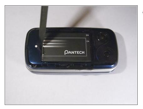
• Carefully lift the battery up from where the spudger is pointed.
