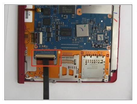
Using the flat end of the spudger, pry open the brown flap that connects the cardholder to the motherboard.
