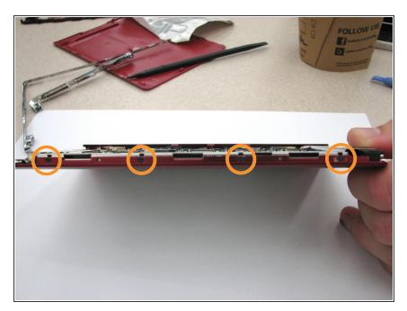
Remove the four 1.4 mm screws that are located on the side of the device that are usually covered by the bottom and side panel.
