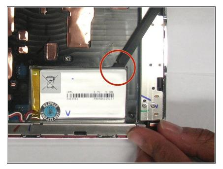
Use the flat end of the spudger to pry the battery out of its holder. There may be glue holding it in place.
