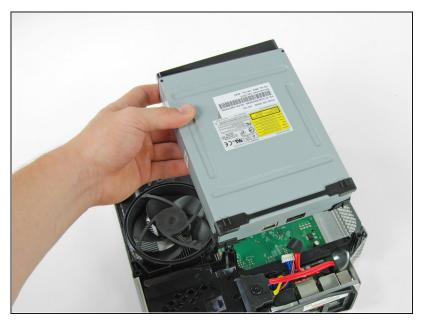
• Lift the optical drive out of the Xbox.
