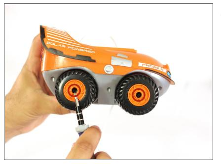
Remove 8.0mm Phillips #1 screws, one for each wheel.
