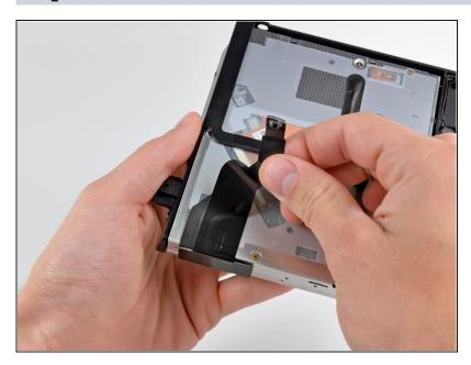
• Peel the optical drive cable off the body of the optical drive.
