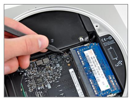
Use the tip of a spudger to lift the IR sensor connector up and out of its socket on the logic board.
