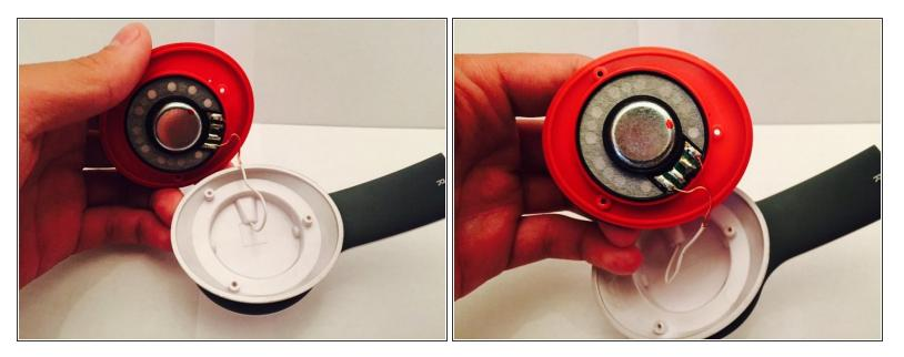
$\bigwedge$  Using safety gloves, desolder the two wires of the speaker.
