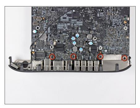
Remove the four 2.6 mm T6 Torx screws securing the I/O bezel to the logic board.
