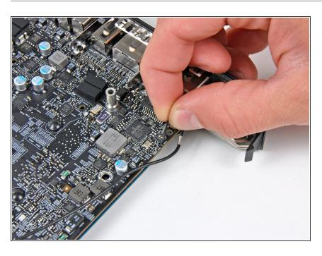
Lift the power button cables upward to gently pull the power button cable up and out of its connector on the logic board.
