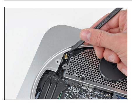
Use the tip of a spudger to carefully pry the antenna connector up off the AirPort/Bluetooth board.
