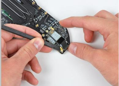
• Use the flat end of a spudger to pry the antenna connectors up off the AirPort/Bluetooth board.
