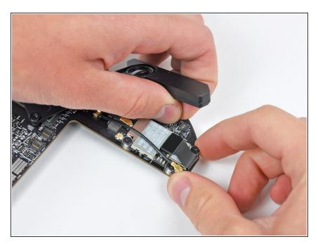
Carefully lift the speaker wires upward to lift the speaker connector up and out of its socket on the logic board.
