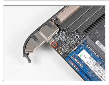
Remove the single 2.6 mm T6 Torx screw securing the I/O bezel to the logic board near the RAM.
