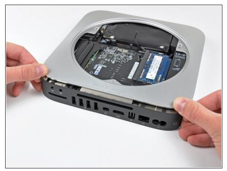
Simultaneously push the two plastic clips on the far left and right sides of the I/O board toward the middle of the I/O board and pull the I/O board away from the outer case.
