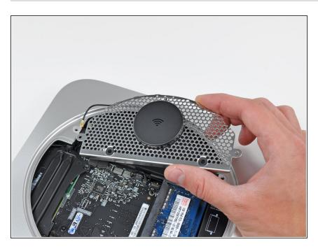
Remove the antenna plate from the mini.
