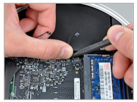
To disconnect the optical drive thermal sensor, pinch its cables between your thumb and a spudger and pry the spudger upward to lift the connector up and out of its socket on the logic board.
