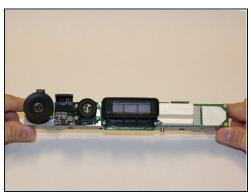
• Lift the motherboard and the heat sink assembly from the plastic shell. The components attached to the heat sink are now accessible.
