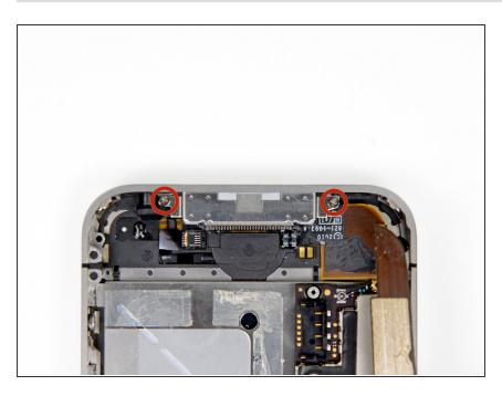
Remove the two 1.3 mm Phillips screws securing the dock connector to the rear case.
