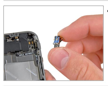
Remove the vibrator from the inner case.
