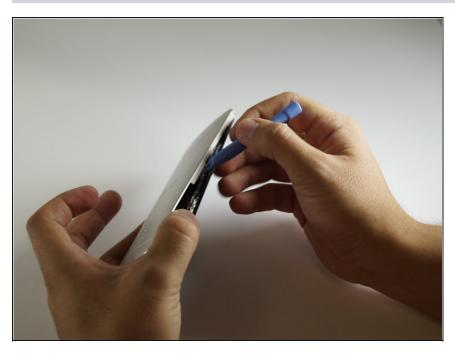
Carefully remove the volume button. Loosen the back panel of the phone with the plastic opening tool. Begin loosening and prying in the space where the battery was.
