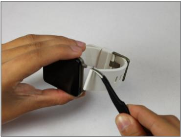
This is a challenging step. Do it carefully to prevent the spring bar from flying out of the wristband.
