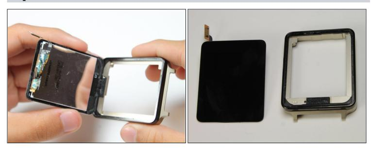
• After using the pick to loosen the adhesive, simply pull the display assembly up from the metal bezel.
