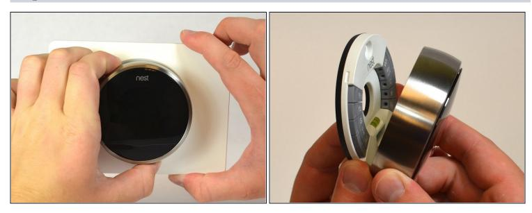
• Grasp the display's metal outer ring with your fingers and pull directly away from the wall.
