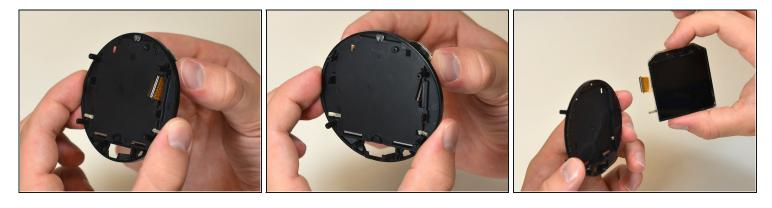
• Pull the LCD screen away from the plastic frame gently using your fingers.
