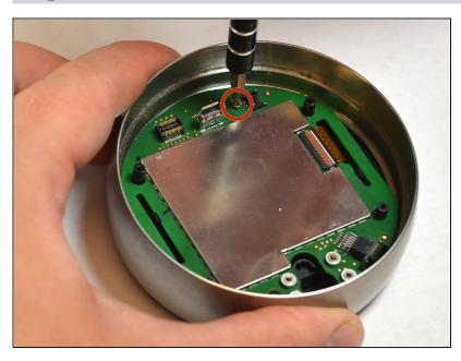
Remove one 4 mm screw from the motherboard using a #0 Phillips screwdriver.
