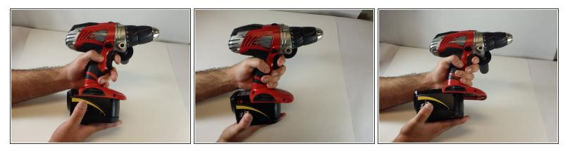
• While holding down the red locking switch, slide the battery towards the back of the drill until the battery is fully removed from the drill.
