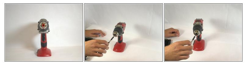
• The chuck sleeve is held on by a 20mm Phillips #2 screw in the center. This screw is reverse threaded. Insert a Phillips #2 screwdriver and rotate it clockwise to loosen and remove it.
