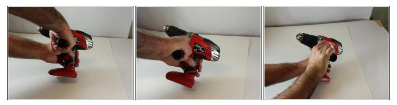
• Grip cordless drill firmly with left hand. Grip the cordless drill handle firmly with the right hand. Rotate the handle counterclockwise in order to remove the handle from the drill.
