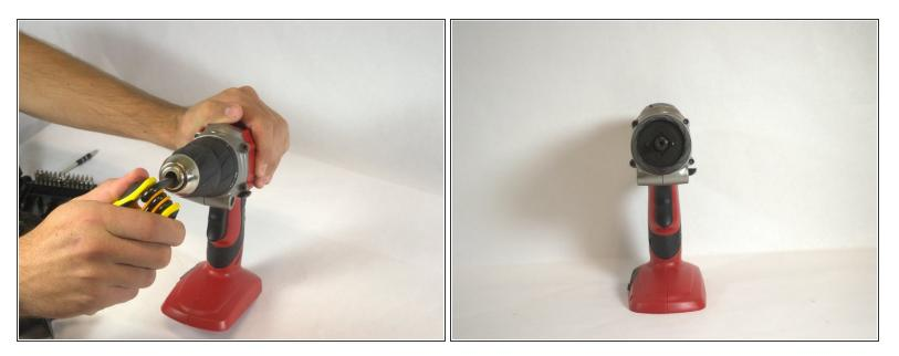
• The threaded hole the screw was in is in the shape of a 6-point star. Insert a T40 Torx Key and rotate it clockwise to loosen and remove the chuck sleeve.
