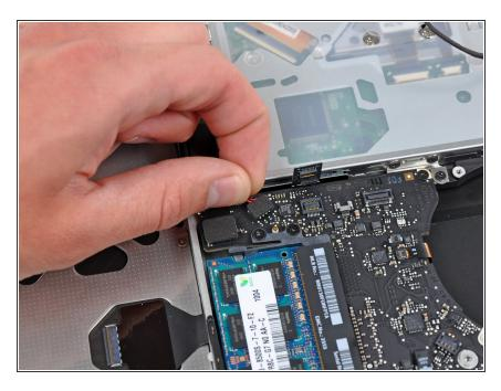
Carefully pull the subwoofer/right speaker cable up to lift its connector out of its socket on the logic board.
