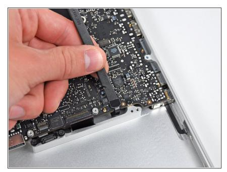
Use the flat end of a spudger to pry the battery indicator cable connector up out of its socket on the logic board.
