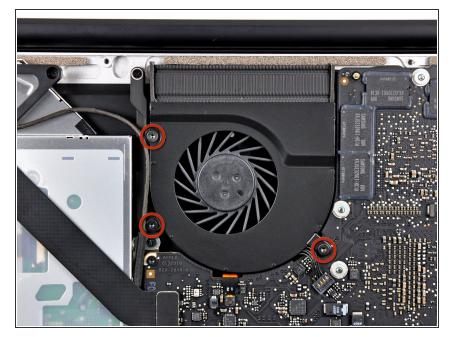
Remove the three T6 Torx screws securing the right fan to the upper case.
