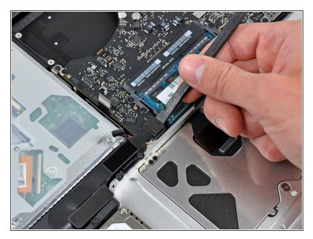
Use the flat end of a spudger to pry the hard drive cable connector up out of its socket on the logic board.
