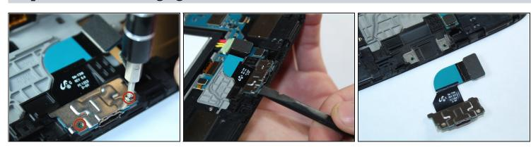
• Unscrew the 2.9mm screws from the charging port with Phillips Head #000 and use the spudger to pry it up from under the port to remove component from the device.
