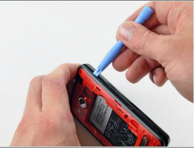
• Insert the iPod opening tool between the rear inner frame and its plastic surround and pry up at several points along the left edge of the Evo.
