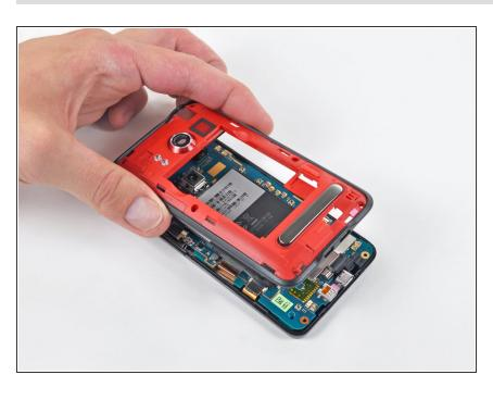
Remove the rear inner frame from the rest of the Evo.
