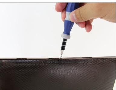
Use T5 Torx Screwdriver to remove two 4.5 millimeter T5 screws on either side of the port on the bottom of the tablet.
