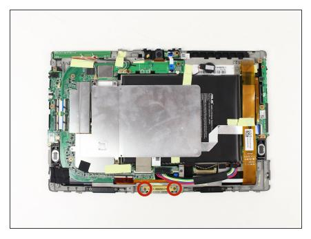
Use a Phillips #00 Screwdriver to remove the two 3 millimeter screws found at the bottom center of the tablet near the charging port.
