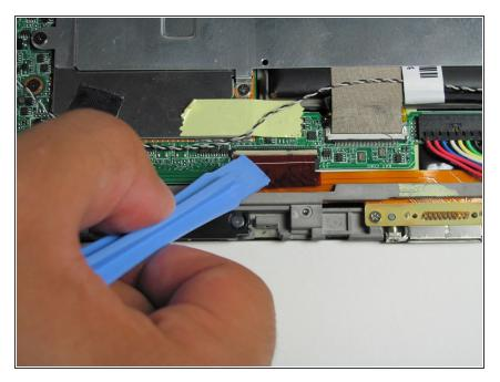
Use Plastic Opening Tool to lift up the white flap found to the left of the charging port.
