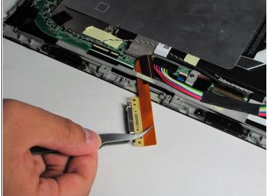
• Use Tweezers to wiggle the port panel out from underneath the metal bar.
