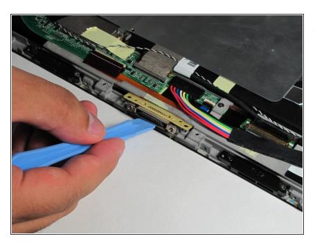
Use Plastic Opening Tool to lift up the charging port.
