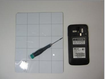
• With your back panel already removed from the previous guide you'll need to acquire a Philips head screw driver size (PH00)
