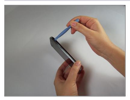
Remove the back cover of the cell phone using a plastic opening tool.
