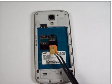
• Using <u>tweezers</u>, remove the SIM card by sliding it towards the bottom of the device.
