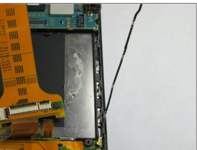
Use the plastic opening tool to unlatch the cord's ends off the motherboard and loud speaker module. The cord can be located on the right side of the phone.
