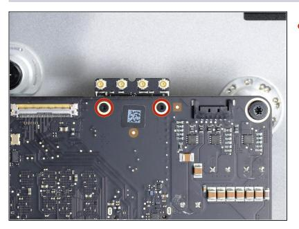
Remove two 3.7 mm T5 screws securing the AirPort/Bluetooth card to the logic board.
