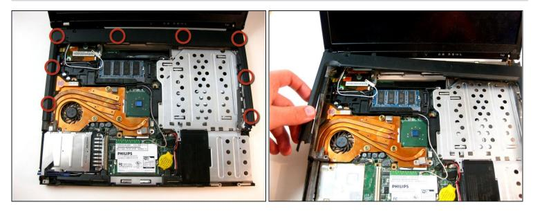
• Starting from the bottom right, carefully pry off the bezel. Use a spudger or flathead screwdriver if assistance is needed.
