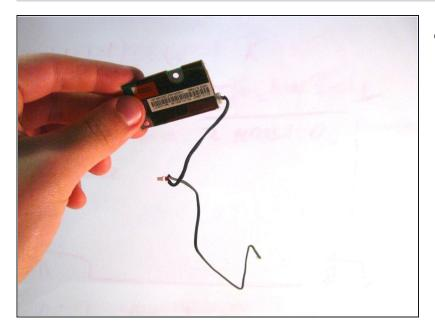
• The cables are routed through different components for organization, carefully disconnect them, unwrap them and pull the card free.
