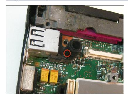
• Remove the rubber cover from the microphone.
