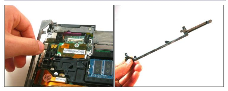
• Grasp the metal bracket to remove it from the device.
